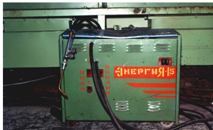
Figure 4. Installation welding hydrogen-oxygen Energy-1.5 UHL – 4.
